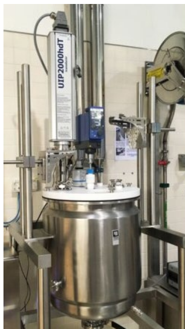
Figure 9. UIP2000hdT ultrasonic homogenizer (2 kW, 20 kHz) for efficient mixing, homogenization, nano-dispersion, nano-emulsification, and extraction, [29]
