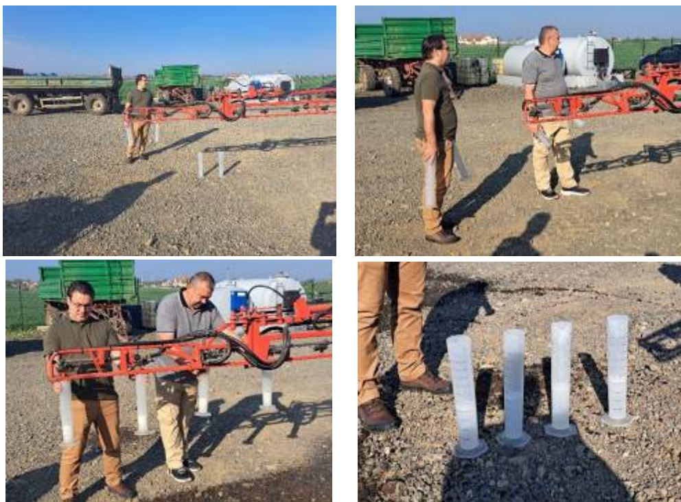
Fig. 12 Determining the flow rate at the red nozzle.
