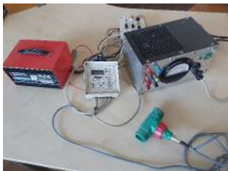
Fig. 7 Flowmeter + flow sensor + Flow measurement device + RAU MULTI-CHECK.
