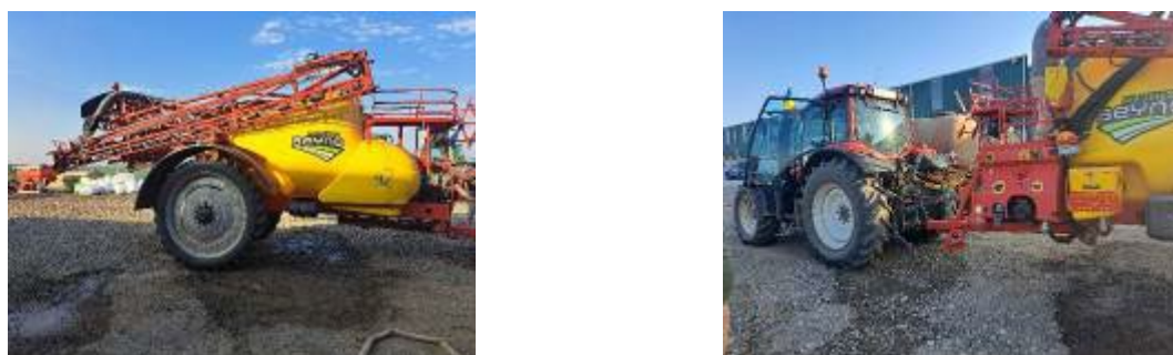
Fig. 9 Beyne sprayer in aggregate with a Valtra tractor.
