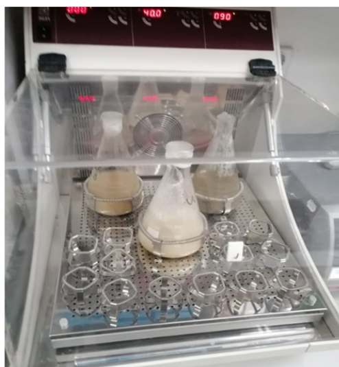
Figure 1. Hydrolysates of raw wool and pelleted wool in the shaking incubator
