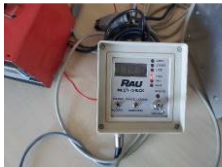
Fig. 7 Flowmeter + flow sensor + Flow measurement device + RAU MULTI-CHECK.
