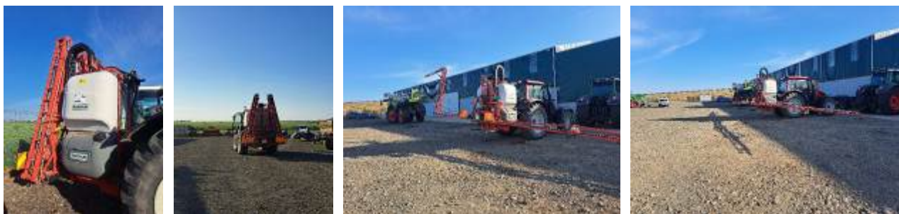
Fig. 3 BARGAM portable sprayer – 1200 [ l ]/ 18 [m]– Caruntu Farm.
